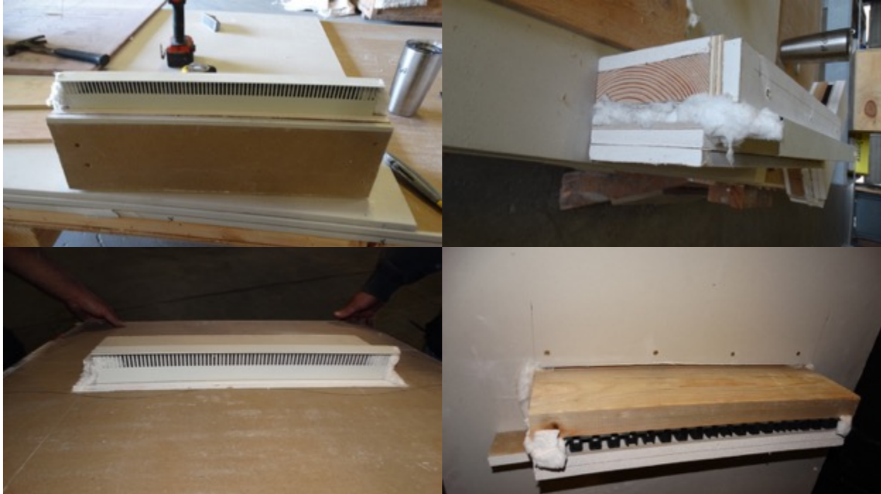
Figure 6. Representative samples showing (a) flashing gap for ember test, (b) side cross-section for ember test, (c) flashing gap for flame test, and (d) crawl-space side of vent system.
