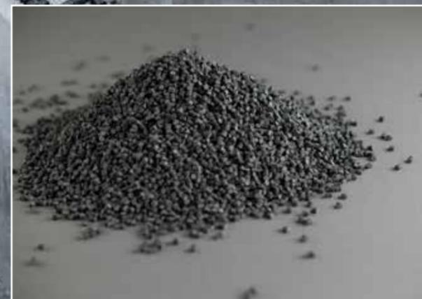
The Joto-Vent is made of "JC (Joto-Compound)", a composite material that consists of calcium carbonate, polyolefin resin and recycled plastics.
