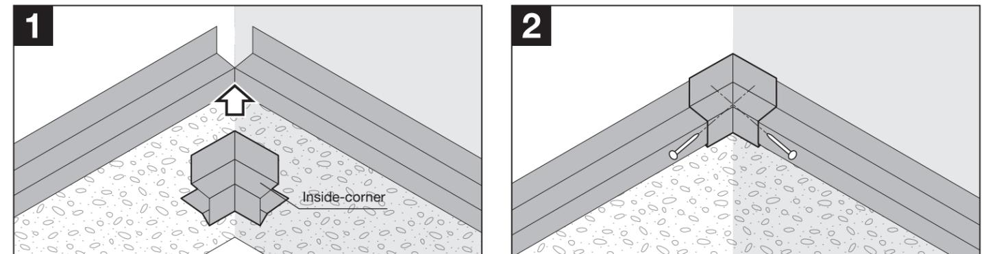
**Joint-cover:** install by using stainless-steel nails as shown in the illustrations.
