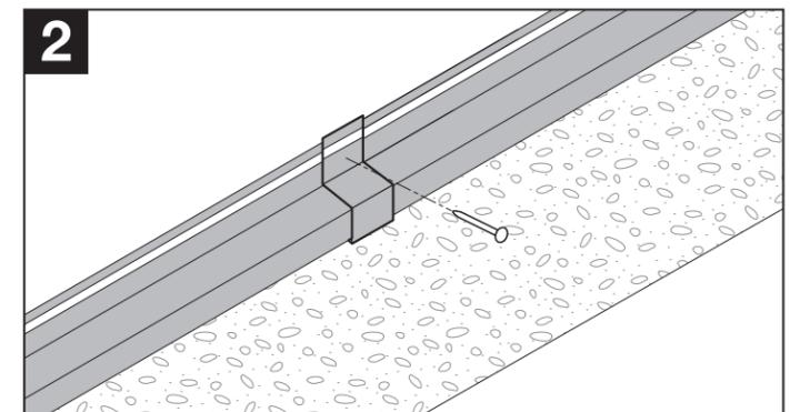
**Endcap:** install by using stainless-steel nails as shown in the illustrations.
