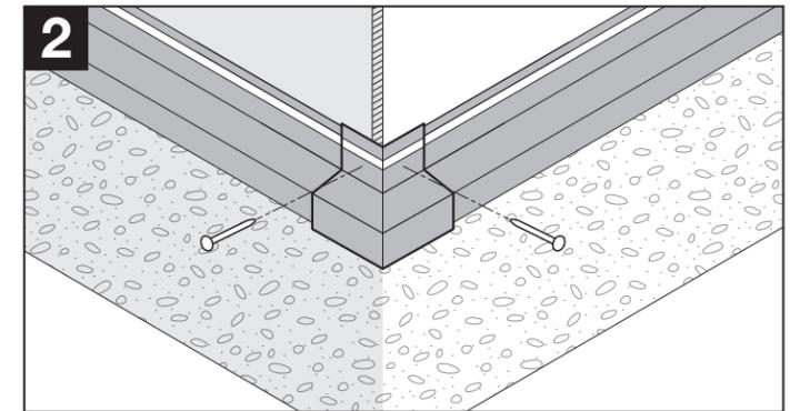
**Inside-corner:** install by using stainless-steel nails as shown in the illustrations.
