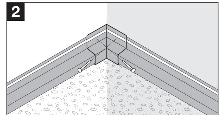
**Joint-cover:** install by using stainless-steel nails as shown in the illustrations.
