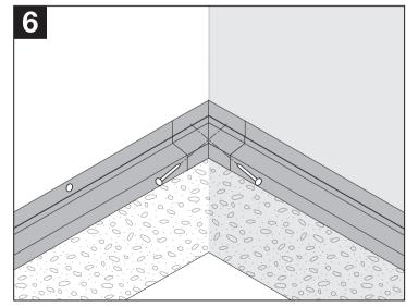
Outside-corner: connect by using joint-pins and install by using stainless-steel nails as shown in the illustrations.
