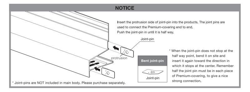
**Joint-pin:** install by connecting joint-pins as shown in the illustrations.
