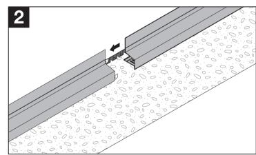
**Endcap:** install by using stainless-steel nails as shown in the illustrations.
